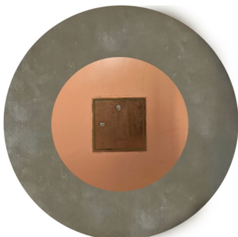
(c) Proposed antenna with the conducting skin.
